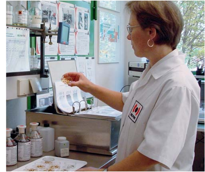
Evaluation of a grey cast iron chip test according to DIN and FED standards
